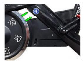
3. Remove the brake pad <sup>(5)</sup> by removing the one mounting bolt using a 3 mm hex key. Retain fastener hardware for installation.
